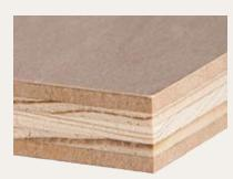
Combi-Core Panels - Constructed of veneer core inner plies with particleboard or MDF cross-bands. Offers similar strength and stability to veneer core but has the void-free surface quality of PBC. (Veneer core inner plies with MDF outer crossbands shown here.) Excellent substrate for the thin sliced woods & even rotary woods, reducing the potential for core transfer. Combi-core panels tend to offer more consistent tolerances than standard veneer cores.
